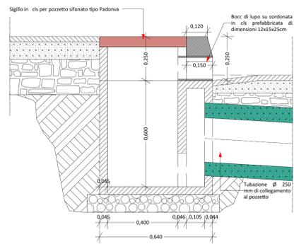
POZZETTO DI RACCOLTA SIFONATO CON CADITOIA IN GHISA SCALA 1:10
